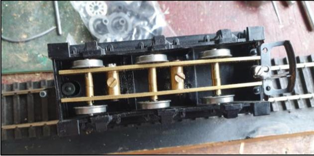
The tender, which should have been simple, was a problem as I could not get replacement wheels to sit square on the original axles. So, I made up a brass frame with 9mm spacers and fitted 6 x 12mm insulated wheels.
